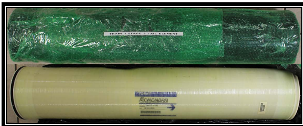
Figure 5: The membrane arrived intact and in good condition.
