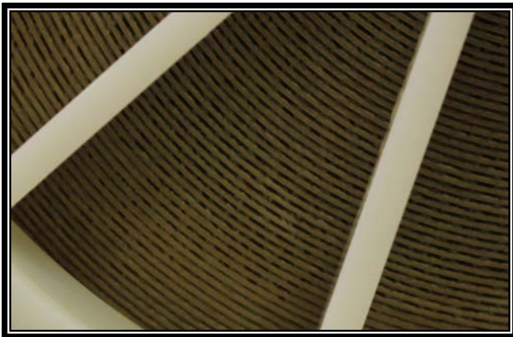
Figure 8: The feed end feed channels were visibly discolored.
