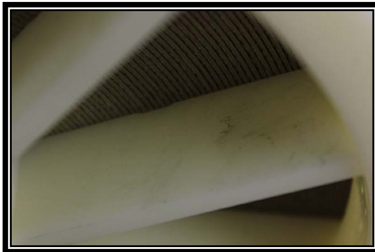
Figure 10: A black deposit was found on a spoke of the concentrate ATD.
