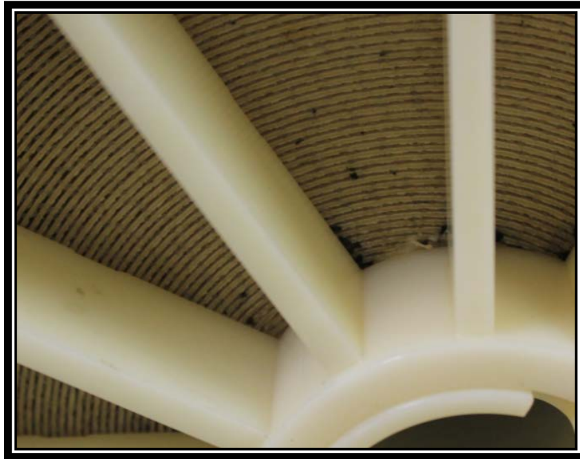
Figure 3 Black deposits were observed in the feed end feed channels.
